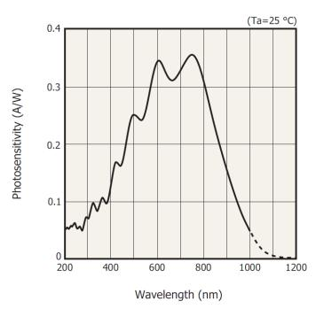
Hamamatsu provides newer versions of their sensors on a regular basis with improved spectral response. Below is an example of the \$12198 (old version) and \$12198-01 (new version) with improved spectral response in the UV:
